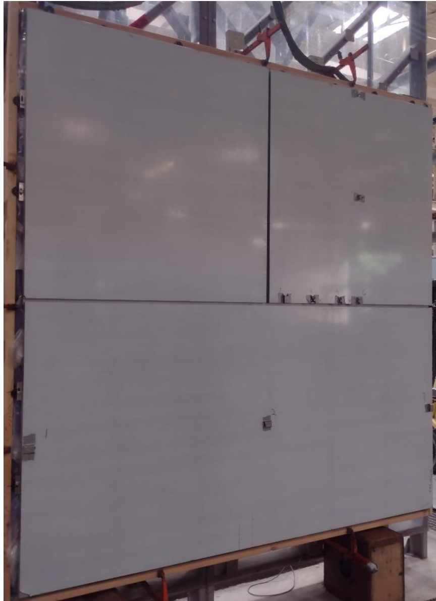
Photo No. 5 etalbond® FR (ACM Panels) Fixed on the EVO™ Rivetless™ Attachment System TAS 202 Specimen #5 prior to Testing
