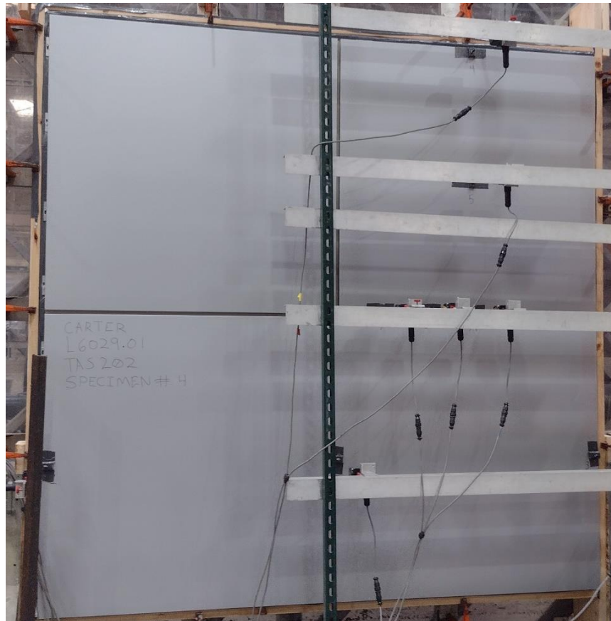
Photo No. 4 etalbond® FR (ACM Panels) Fixed on the EVO™ Rivetless™ Attachment System TAS 202 Specimen #4 Prior to Testing
