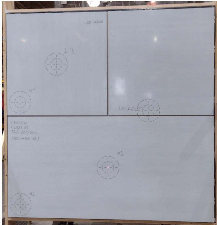
Photo No. 1 etalbond® FR (ACM Panels) Fixed on the EVO™ Rivetless™ Attachment System TAS 201 and TAS 203 Specimen #1 Prior to Testing
